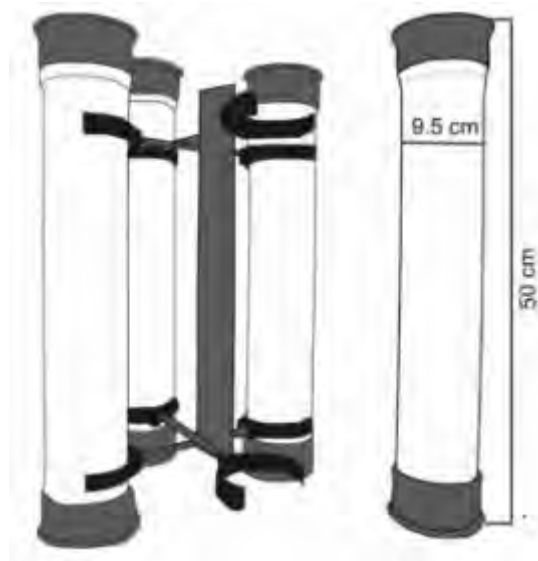
Figure 7.10: Example of a sediment trap instrument (taken from Szmytkiewicz et al 2014).
